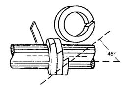
If the butt cut rings are cut on a flat surface, be certain that the side of the master rings, and not the O.D. or I.D. surface, is laid on the rings to be cut. This is necessary so that the end of the rings can be reproduced.
