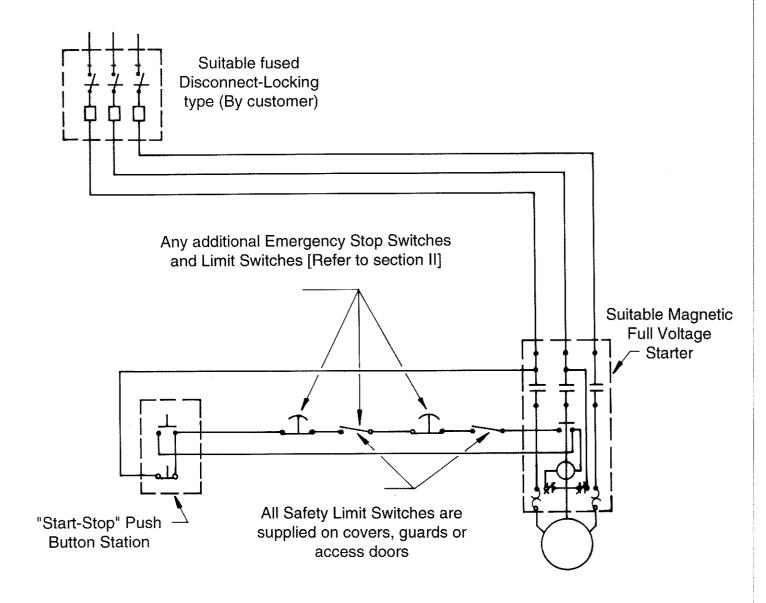
**Note:** Be sure all wiring and components comply with applicable Federal, State and local regulations as well as current national safety standards.
