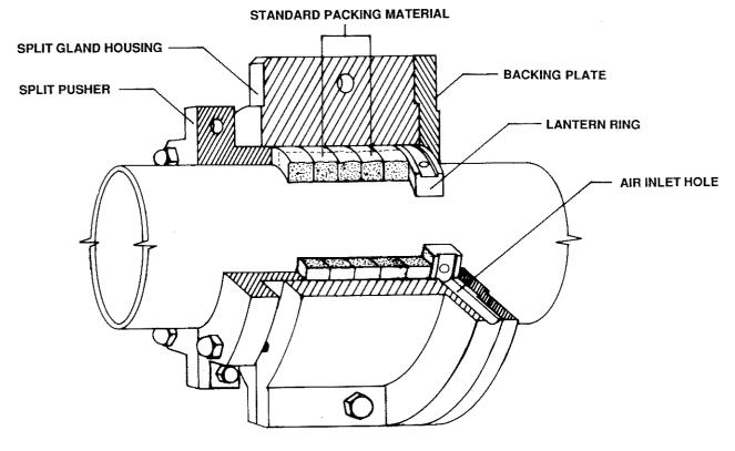
The purpose of the Lantern Ring is to prevent the product from getting inside the gland. This gland was developed primarily for sugar based products. By putting a positive air pressure on the Lantern Ring (3-5 lb./sq. inch) a constant flow of air comes out the inside and does not allow the product in.
